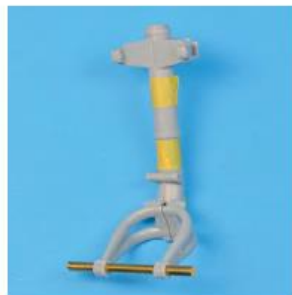
▲ The nose wheel fork was drilled through, and brass rod formed the axle so the wheel could be fitted after the gear was painted and weathered.
