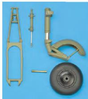
▲ The nose wheel fork was drilled through, and brass rod formed the axle so the wheel could be fitted after the gear was painted and weathered.
