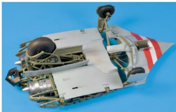
▲ The bottom of the fuselage was weathered with ground pastels applied by micro-brush, while fasteners received a Payne's Grey pin wash to accentuate them.
