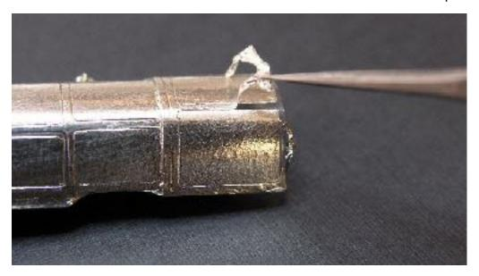
being methodical and using only light pressure on the blade. With its recessed frame lines the Hasegawa canopy was very easy and simple to cut. The blade stayed right in the groove. The rounded corners of the framing were a bit tricky, but I found that placing the blade on its tip and going slowly to be the best method for this kind of cut.
